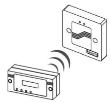
The Card Simulator allows adding and removing any card/card number from the reader memory when the card is lost or not available. One unit can be utilized at different sites but for security reasons it will operate only in conjunction with the Master Card.
